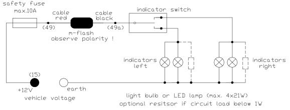
Attention! The minimal supply cable width is 0,75mm<sup>2</sup>. You must fuse the +12V power supply cable with a 10A safety fuse. If the device will be used without fuse, damage at the connecting cable or the m-flash itself can cause a shortcut and a cable fire. There may be a risk of your life! If you are not capable to connect the device properly, let the professional motorcycle technician do the job.
