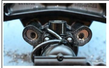
Drill out breakaway screw and remove ignition lock from OE triple clamp. Use a 6mm drill bit (or ¼" if no 6mm drill bit is around)
