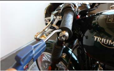
Remove left handlebar grip with air pressure.
