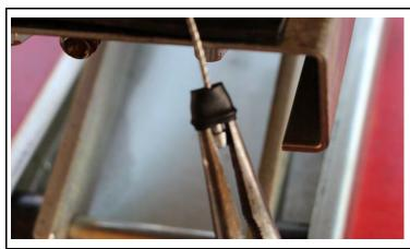
Remove the protective rubber from the original cable and slide it over the new one.
