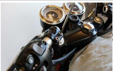
... from the clip-on handlebars; in doing so pull the headlight cable completely out of the headlight housing.
