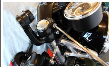
Loosen the clamping bolts of the triple clamp and clip-on clamps on the fork leg.
