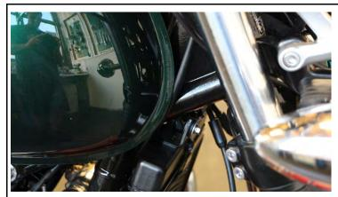
The new clutch cable will be routed over the radiator fan from the left to the right side...
