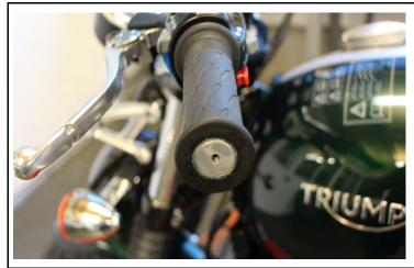
Glue left rubber grip flush to the handlebar bushing. Use glue in reference to your Triumph manual.
