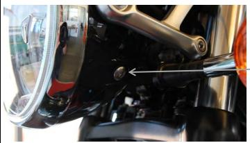
Remove both mounting bolts for the head light.
