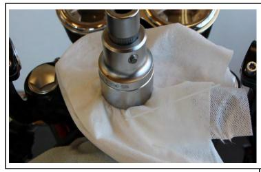
Loosen steering stem nut on the upper triple clamp. (Use cotton rag to avoid scratching the triple clamp)
