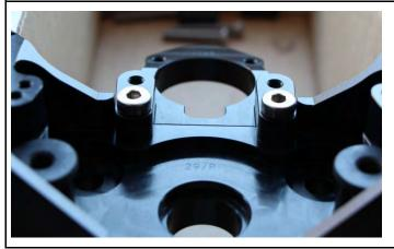
Mount the speedo bracket using the M8x20 bolts to the new triple clamp; torque 22Nm (16 ft lb). Loctite blue is always a good idea!
