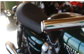
Drive both press bushings with a polyurethane hammer into the handlebar (countersunk to outside).
