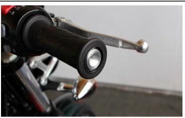
Install right switch housing. The throttle tube should be flush with the handlebar bushing. For the final install of the switch housings it is necessary to drill holes into the handlebar for the locating pins (not for all models). Therefor wrap 1-2 layers of electrical tap around the handlebar (where the locating pins would be), align the switch housings and press onto the housings. Next center punch the marked positions and drill accordingly to the locating pin diameter.
