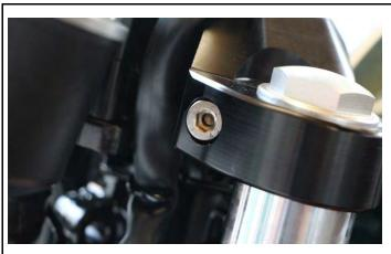
Position triple clamp completely over the fork legs.
