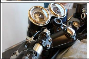
Loosen up the clip-on bar screws subsequently removing the safety and clip-on bars.
