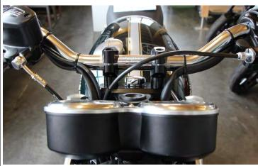
Remove the original clutch cable and replace it with the new one.
