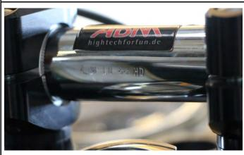
Install switch housings and clutch/brake/throttle onto the new handlebar.
