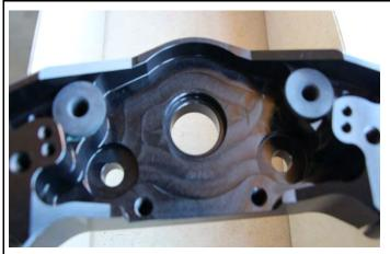
Remove rubber grommets from the OE triple clamp and install them into the new triple clamp.
