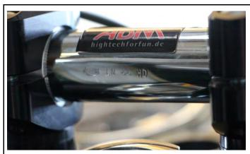
Install the riser clamps (BK1R) and 15mm spacers to the triple clamp (torque 30Nm, 22 ft lb).
